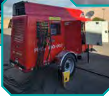
◀ Fuel Booster Pump Modification installed in SAFER 480V Turbine Generators
