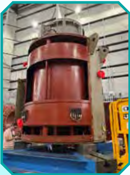
▲ Contaminated Reactor Recirc Pump Motor received by PIM as replacement motor for rotating spare EC.
